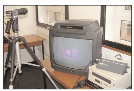
Typical installation with CCTV Camera, monitor and VCR
